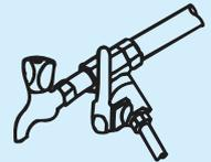
5. Now connect one end of the pipe to the SS ball valve and other end to the elbow fitting connector labeled as WATER IN, on the left side of purifier.
