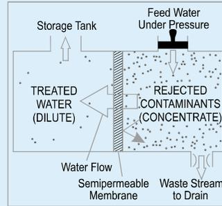
The rejected impurities on the concentrated side of the membrane are washed away in a stream of waste water and thus do not get accumulated, as in a traditional filter.
