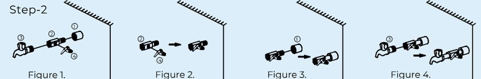
1. First fix the SS ball valve (marked as no. 4) to the 1/4 inch port of the 3-way connector (marked as no. 2) as shown in figure 2.
