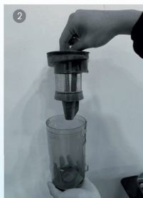
Take over the filter and metal filter from dust cup.
